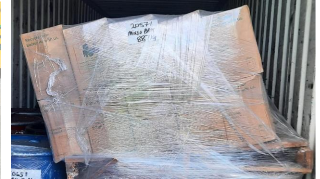
How Not to Stack Cartons ✗
