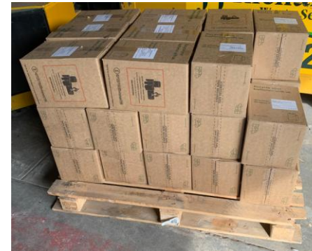
How Not to Stack Cartons ✗
